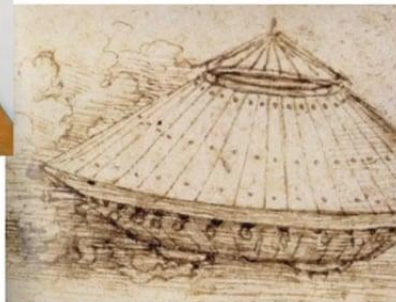
A sketch for an armoured vehicle like that could move in all directions
