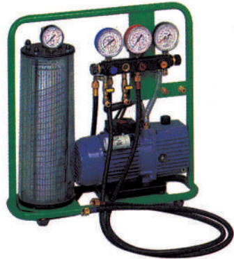
Portable charging equipment (Vacuum pump, charging cylinder, gauge test set and hoses)
