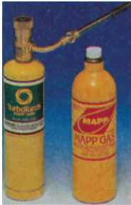
Portable MAPP gas bottles suitable for gas soldering or brazing
