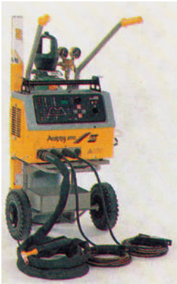
Machine used for electric brazing and welding
