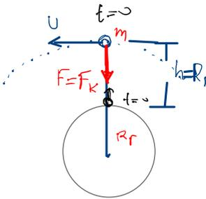
4.4)  $v = \frac{2\pi R}{T} \Rightarrow T = \frac{2\pi R}{v} = \frac{2\pi(R_\Gamma + h)}{v} = \frac{2\pi 2R_\Gamma}{v} = \frac{4\pi R_\Gamma}{v} = \frac{4\pi \cdot 64 \cdot 10^6}{4\sqrt{2} \cdot 10^3} = \frac{64\pi}{\sqrt{2}} 10^3 \Rightarrow T = \frac{64\pi}{\sqrt{2}} 10^3 \Rightarrow$
