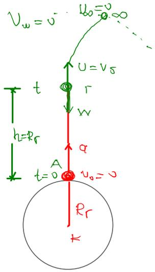
$$\frac{1}{2} v_\delta^2 = \frac{GM_\Gamma}{2R_\Gamma} \Rightarrow v_\delta^2 = \frac{g_0 h^2}{R_\Gamma} \Rightarrow v_\delta = \sqrt{g_0 R_\Gamma} = \sqrt{10 \cdot 10^5 \cdot 64} = \sqrt{64 \cdot 10^6} = 8 \cdot 10^3 \Rightarrow \boxed{v_\delta = 8 \cdot 10^3 \text{ m/s}}$$
