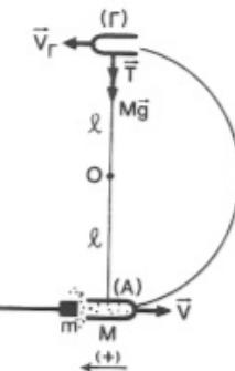
$$\text{α)} \text{ Ενεργή } \sum F_{\text{αντ}} = 0 \Rightarrow \text{Ισχυρ } \text{ στ } A.D.O : \vec{P}_{0x} = \vec{P}_{0x} \Rightarrow mu - MV = 0 \Rightarrow V = \frac{m}{M} u = \frac{4}{20} 30 = 6 \text{ m/s}$$
