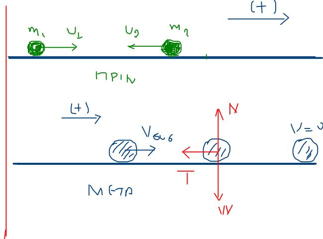
$$\text{α)} \quad P_1 = m_1 v_1 = 6 \cdot 20 = 120 \text{ kg m/s} \quad P_2 = m_2 v_2 = 4 \cdot 10 = 40 \text{ kg m/s} \quad \Rightarrow V_{6v6} \text{ προς τα θερινά, Πρόρρηματι στον άδειο: } \vec{P}_{02} = \vec{P}'_{02} \Rightarrow \\ (m_1 + m_2)V_{6v6} = m_1 v_1 - m_2 v_2 \Rightarrow V_{6v6} = \frac{80}{10} = \boxed{V_{6v6} = 8 \text{ m/s}}$$
