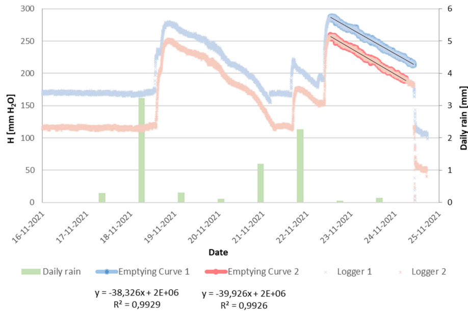
Fig. 9. Infiltration curve results for the Kaczeńce rain garden (two loggers).
