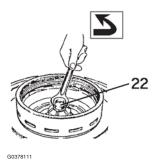
Fit sliding bowl bottom (21). Make sure that the square seal ring lies concentrically in its groove. Press the sliding bowl bottom down on the upper distributing ring.
