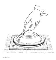
Removal of seal ring on sliding bowl bottom.
