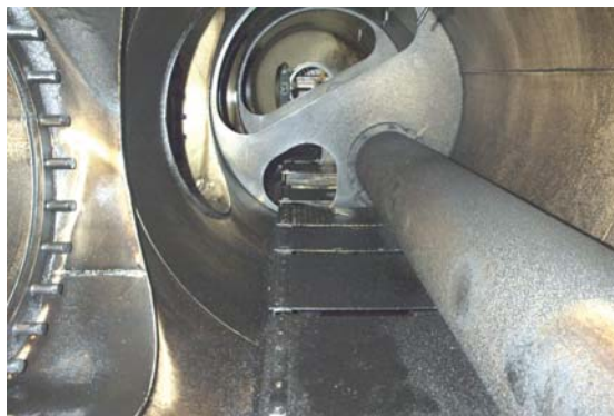
Scavenge Receiver, MUCH SLUDGE - MS
