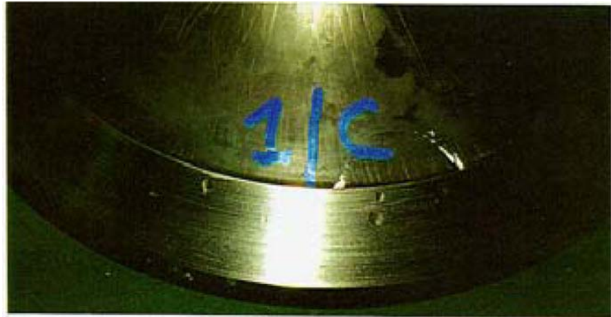
Photo 5: Acceptable seat condition after grinding
