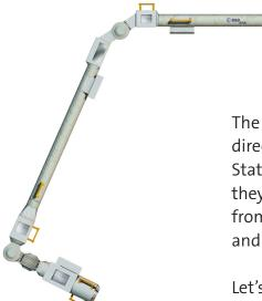
The European Robotic Arm will move small payloads directly from inside to outside the International Space Station. It will also move astronauts to a position where they can work on the exterior of the Space Station , or from one external location to another. This saves time and effort during spacewalks.
