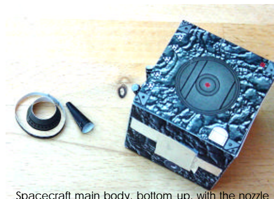
Spacecraft main body, bottom up, with the nozzle of the main engine, the separation ring and the nozzle protection on the left
