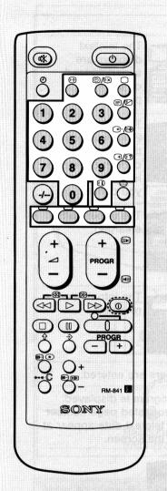
TV stations broadcast teletext programmes via the TV channels. To receive teletext programmes, use the buttons indicated in green on the Remote Commander.
