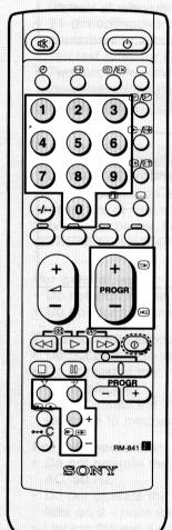
After having installed the TV, you now need to preset TV channels. Up to 60 programme positions are at your disposal. For channel presetting use the buttons with the red symbols on the Remote Commander.
