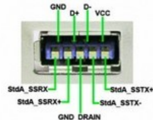
SuperSpeed standard A plug pinout
