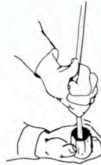
25. Removing burrs from tubes
