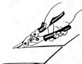
16. Shearing thin sheets of metal
