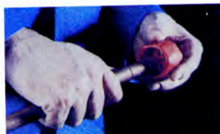
Removing the burrs with a reamer
