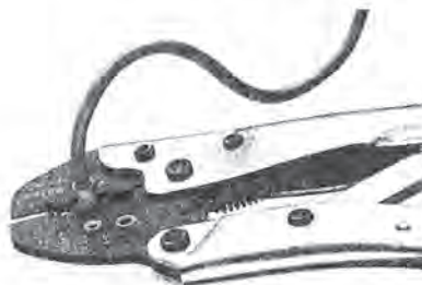
10. Crimping terminals to cables and wires
