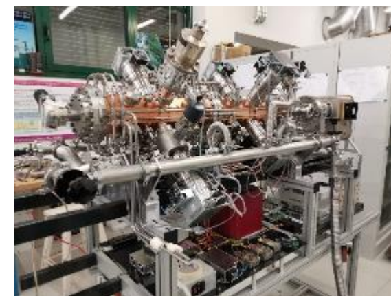
Portable PIXE system based on an RFQ linac being built by CERN and LABEC
