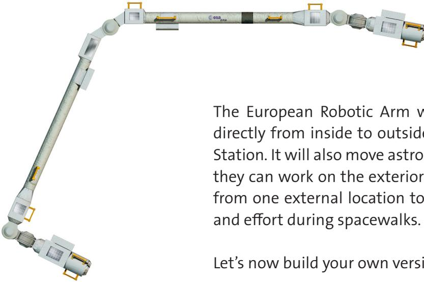
The European Robotic Arm will move small payloads directly from inside to outside the International Space Station. It will also move astronauts to a position where they can work on the exterior of the Space Station, or from one external location to another. This saves time and effort during spacewalks.
